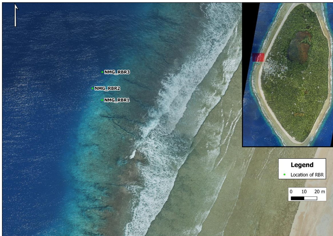
Figure 16: Deployment of RBR tide and wave recorders on Nanumaga.
