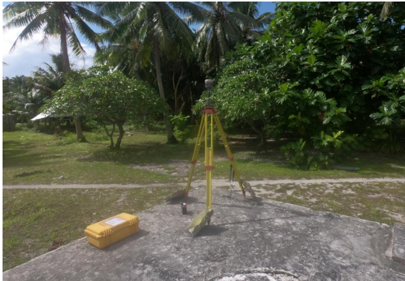
Figure 10: Set up of a base station over a bench mark in Niulakita for GNSS observation.
