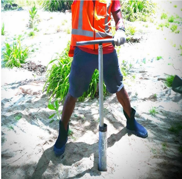
Figure 4: Hand auger and casing.
