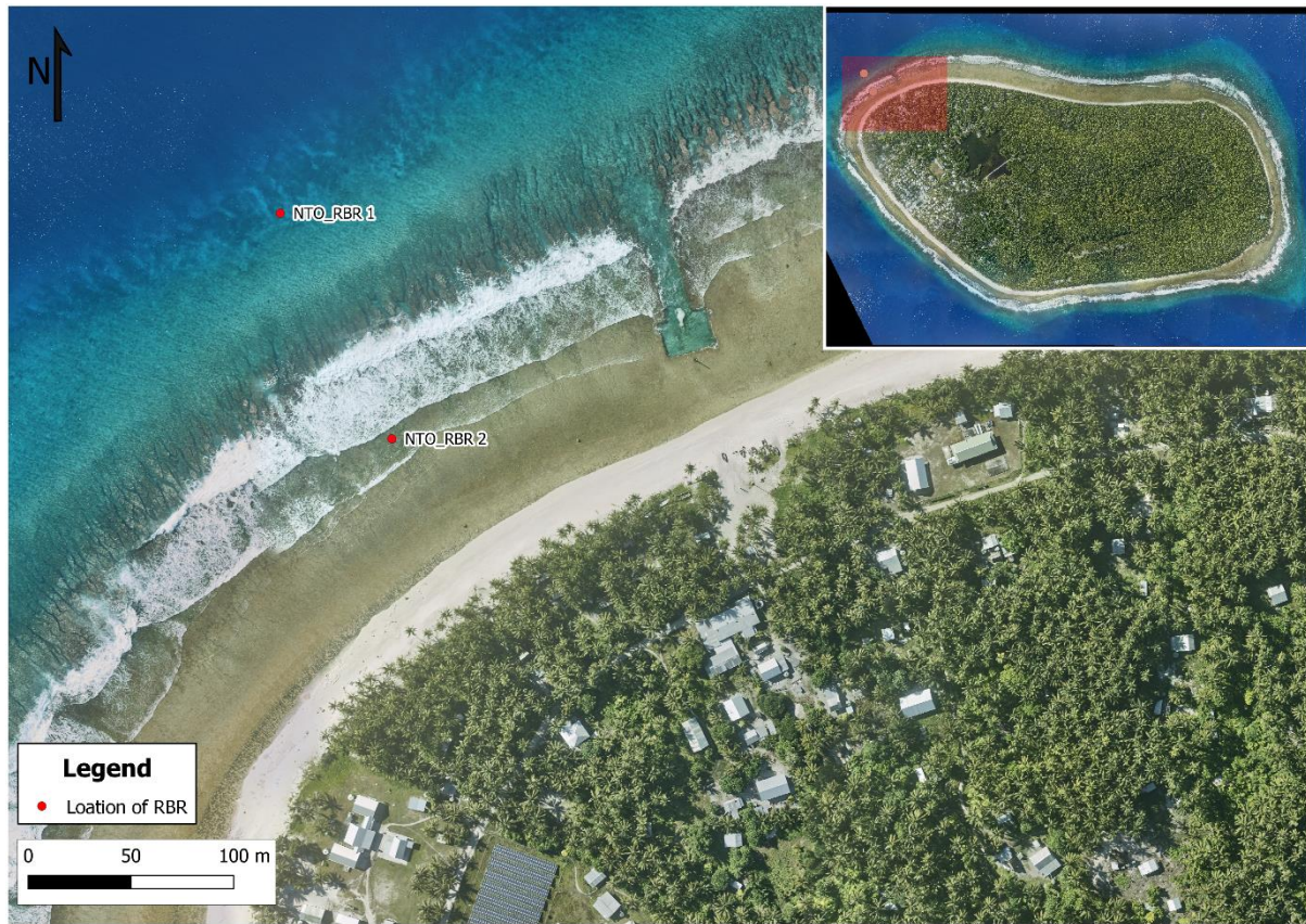
Figure 20: Deployment of the RBR tide and wave recorders on Niutao.
