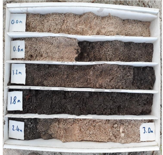
Figure 5: Example of hand auger sample placed in core box.
