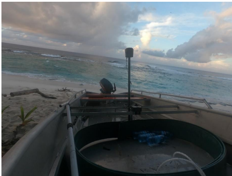
Figure 11: GNSS receiver installed on fishing boat, ready for pole to gauge calibration
